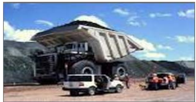
Fig. 1: A dumpers used in an open cast mine
